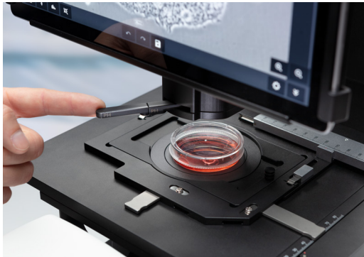
Move the contrast slider easily to switch between phase contrast and brightfield.
